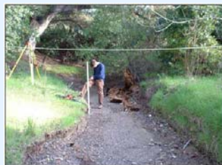
Figure 3-4 Cross-section survey at YB1-4. A tape was stretched between two pins to measure the channel dimensions, bed material, bank material, vegetation, roughness and other characteristics were described.
